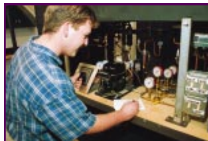
Brian Phillips (Calif.) takes readings from thermocouples on a heat pump.
